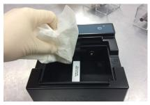
1. Wipe up any moisture from the inside of the carriage and around the rivets as soon as you are done.
