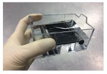
Rinse the tank, gel tray, and casting stand with deionized or distilled water.
