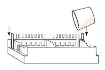
4. Carefully remove comb when gel is ready. Remove gel tray with solidified gel from casting stand and wipe off any excess agarose from the bottom of the tray.
