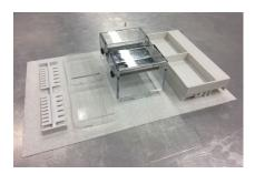
3. Allow the tank, gel trays, and casting stand to dry upside down.
