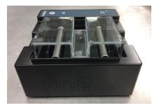
Store the tank upside down inside the carriage. This relieves pressure on the connectors.
