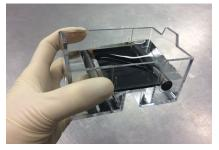
Rinse the tank, gel tray, and casting stand with deionized or distilled water.
